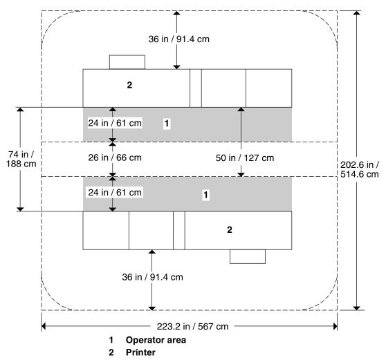
**Face-to-back shared space** The following figure shows the two printers arranged with one facing the back of the other. Between them is 60 inches / 152.4 cm of space. This allows for 24 inches / 61 cm of operator space in front of the printer facing *toward* the other, plus 36 inches / 91.4 cm of service space behind the printer facing *away from* the other.
